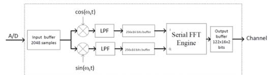
Figure 3: Xampler block diagram.
