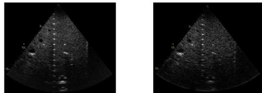
Figure 4: Ground Truth Phantom image (left) Vs. image reconstructed from low rate wireless data (right).
